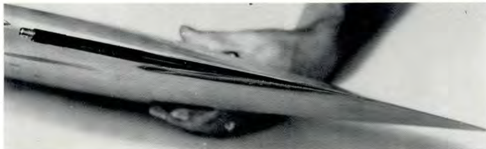
Above, the initial contact point of the lightning was on the screw heads. Note burned fiber glass. Below, left, a pencil inserted into the fiber glass antenna housing shows 10-inch split. Below, right, lightning also burned 2-inch hole in metal antenna.
